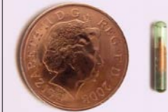
The microchip which is inserted under the skin is smaller than a one pence coin
